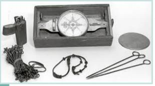
Gunter's Chains were the typical tools the pair of surveyors would use to measure distance and calculate acres of land. In 1620 it was created by Edmund Gunter, a mathematician and astronomer. The actual metal chain was 66 feet long and made of 100 links with each link measuring 7.92 inches. Ten square chains equal one acre and 80 chains equal a mile. The chain was originally called an "acre's breadth" because it was the width of an acre, while a furlong was the length.
